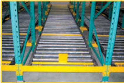
GRAVITY FLOW RACKING
